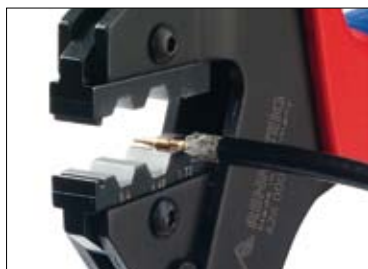
Innenleiter-Crimp Inner conductor crimp
