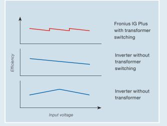
**MIX<sup>™</sup> concept.** You will get the maximum power harvest out of partial load ranges, e.g. on cloudy days, through a clever combination of multiple power stages in each inverter. The power stages in the Fronius inverters divide up the work depending on the operating hours.
